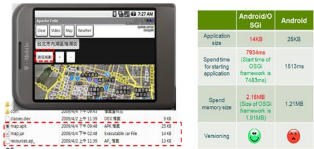
Fig. 12 Lightweight navigation application for Android/OSGi platform
