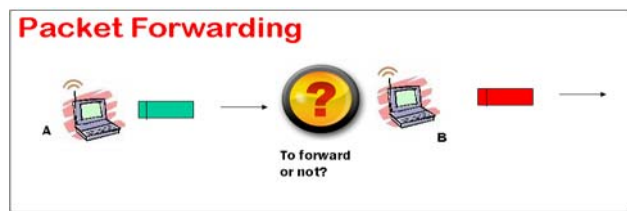
Figure 2. Nodes that are constantly unwilling to forward packets for others may be regarded as exhibiting "selfish" behaviour in an ad hoc mobile network.
