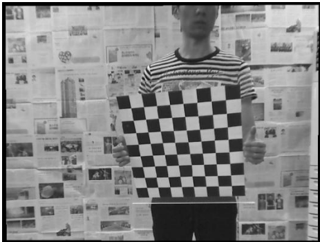
Figure 3. Rectification scene using conventional structure based on 3D sensing stereo camera.
