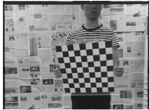
Figure 4. Rectification scene using Newly proposed structure based on 3D sensing stereo camera.
