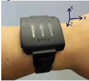
Figure 2. A watch-type human activity detector including a 3-axis accelerometer
