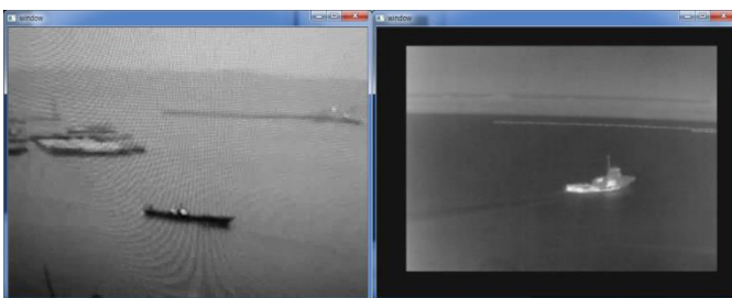
Figure 6. Initial image converted to monochrome information from Figure 2, having same depth but different channel from 3 to 1.
