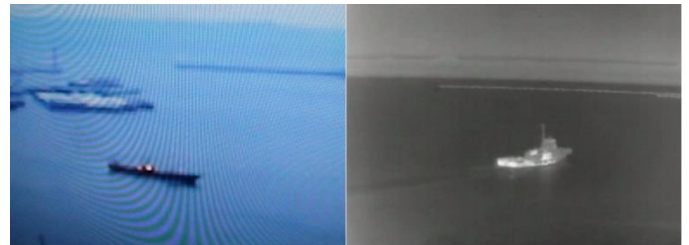
Figure 2. Two initial input images from a CCTV, the left is colour by a CCTV and the right is grayscale by an infrared camera.
