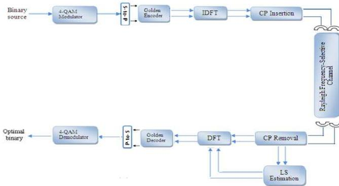
Fig. 2. Block diagram of Coded ASTC-MIMO-OFDM system
