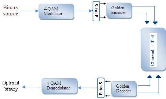
Fig. 1. Block diagram of Coded ASTC System
