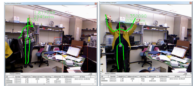
(c) Height and distance detection using Kinect in normal mode
