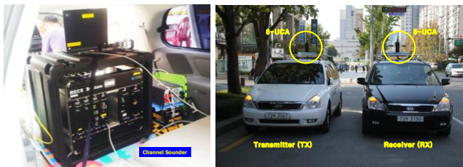
Fig. 1. Installation of channel sounder system and antennas (mounted on the rooftop of vehicle) for channel measurement campaign
