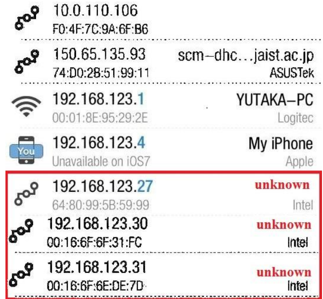
Fig. 10. MAC address spoofing feature of Tails
