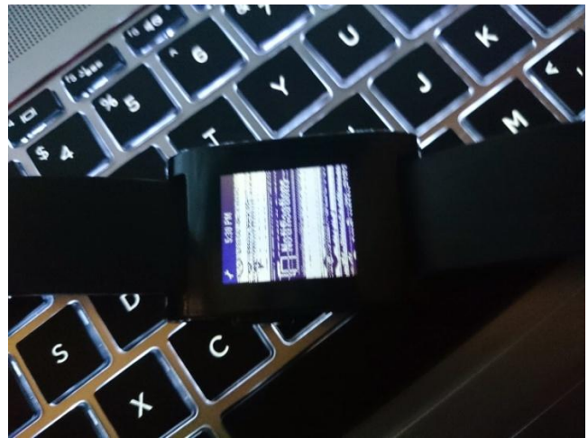
Fig. 1. After DOS attack, the Watch's screen is full of white straight lines, all data and applications are erased because of reset to factory setting [6].
