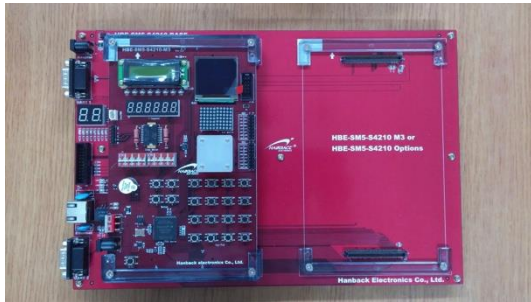
Fig. 5. Multiple sensor module embedded system
