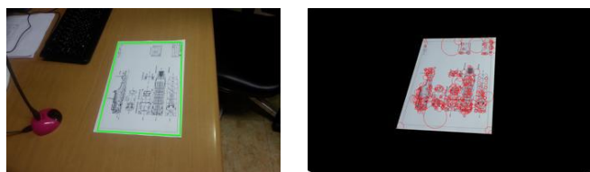
(a) Drawing Region ROI detection (b) Feature points extraction Fig. 10. Feature points matching for design drawings
