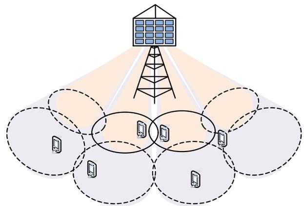
Fig. 1. Multiple beamforming zones using 3-dimension beamforming.
