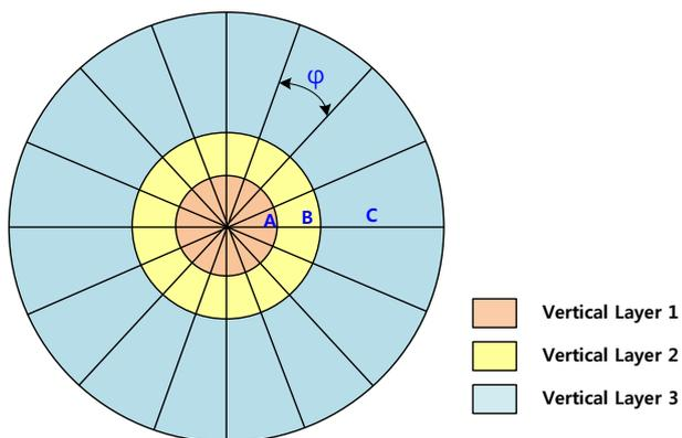
(b) Horizontal view of beamforming layers
