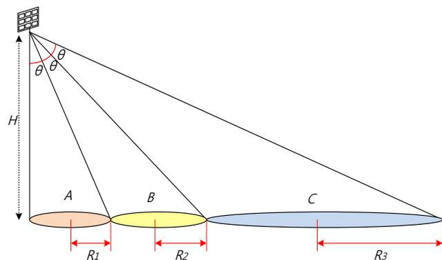
(a) Vertical view of beamforming layers
