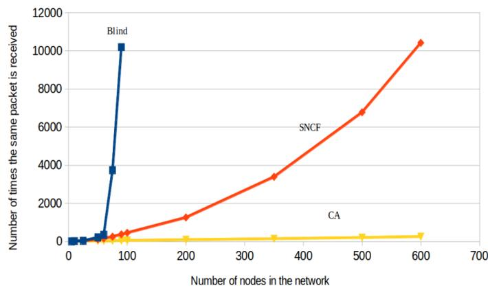
Fig. 3. Performance of Cellular Automata based Rebroadcasting (CA) protocol compared with Blind Rebroadcasting (Blind) and Sequence Number Controlled Flooding (SNCF)
