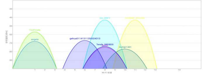
Figure 8. PU instantaneous measurement 2.4G ISM band spectrum
