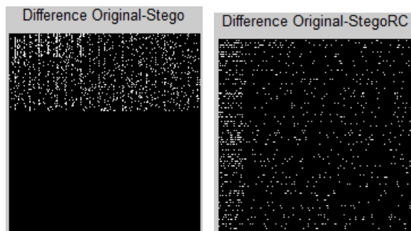
Fig.10. Positions of the embedding changes on non-permuted image (left) and rows and columns permuted image (right) when 0.2 bpp (bit per pixel) is embedded in ‘28.pgm’.
