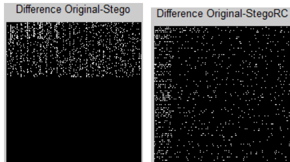
Fig.10. Positions of the embedding changes on non-permuted image (left) and rows and columns permuted image (right) when 0.2 bpp (bit per pixel) is embedded in ‘28.pgm’.
