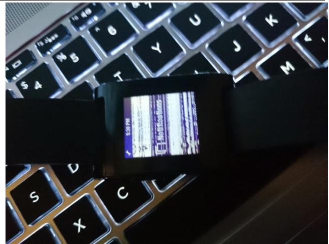
Fig. 5 After DOS attack, the Watch’s screen is full of white straight lines, all data and applications are erased because of reset to factory setting (Hemanth Joseph, August 2014)
