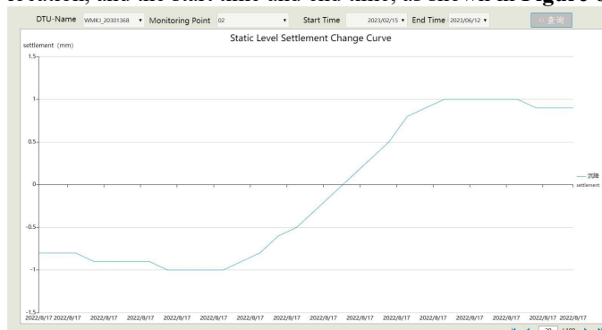
Figure 6. Static level settlement change curve
