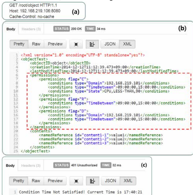
Fig. 10. (a) HTTP request to retrieve a web resource located at '192.168.219.106:8080/root/object/'; (b) HTTP response with successful retrieval of the requested resource; (c) HTTP response with a status code 401 ('Unauthorized')
