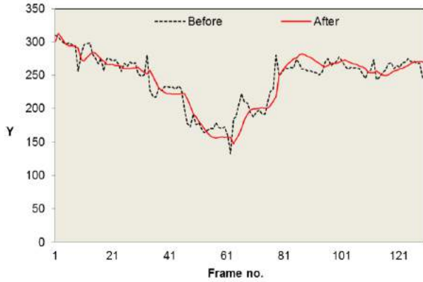
Fig. 6. An application of Kalman filter (parameters Q=0.001 and R=0.0001 )
