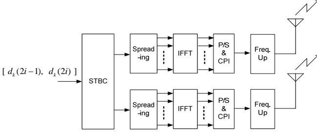
Fig. 1. Transmitter structure for MC-CDMA system employing STBC
