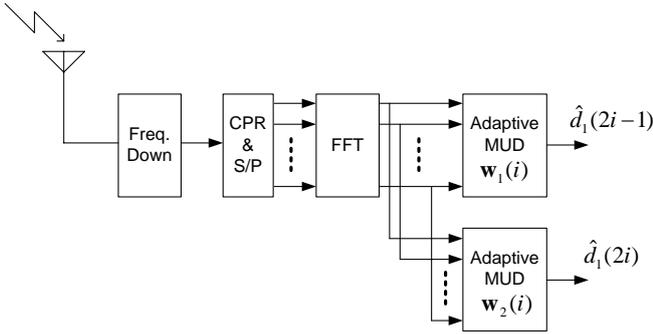
Fig. 2. Receiver structure for MC-CDMA system employing STBC
