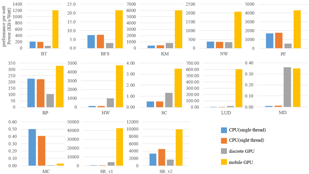
Figure 2. Performance per watt of the benchmarks on the three computing platforms.
