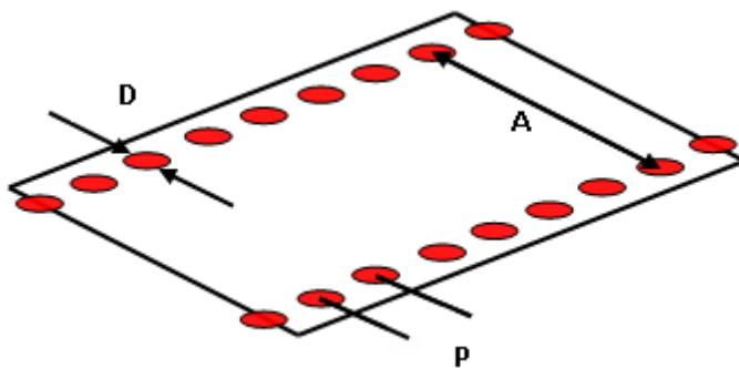
Figure 2. Rectangular wave guide integrated into a substrate.
