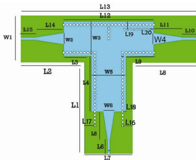
Figure 3. Geometry of the phase shifter.
