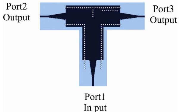
Figure 1. Structure of phase shifter.
